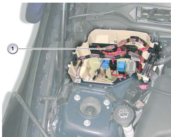
E-box in Engine Compartment (left)
