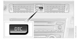
Press the button for at least 3 seconds; the indicator lamps for DSC in the instrument cluster light up. Dynamic Traction Control DTC and DSC have been simultaneously deactivated. Stabilizing and drive-output promoting actions are no longer executed.
