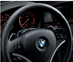
Steering wheel-mounted paddle shifters provide sportier manual gear shifts without the use of a clutch. When equipped with STEPTRONIC automatic transmission and the M Sport Package, paddle shifters are automatically added. In the 335is, paddle shifters are included with the 7-speed Double Clutch Transmission.
