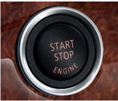
■ Engine Start/Stop button 1 and key fob control the engine. Upon inserting the key fob into the starter switch slot, and the electronic identification system confirms that it is the correct key fob, the engine can be started (or later, shut off) by pressing the Start/Stop button.
