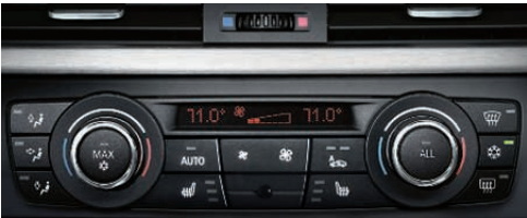
■ Automatic climate control system allows occupants to select a specific cabin temperature and choice of fan speeds, as well as automatic or manual airflow and recirculation. The automatic recirculation control activates whenever certain air pollutants are detected. The system also includes defrost/demist and MAX A/C functions.
