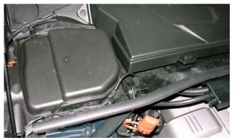
E-box Cover, AUCII Sensor, and Microfilter Housing
