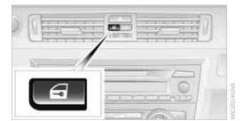
This button serves to unlock or lock doors and the trunk lid, but does not activate the anti-theft system. The fuel filler flap remains unlocked.
