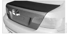
Press the button, see arrow, or the was button on the remote control for a longer period. The trunk lid will open slightly. It can now be swung upwards.
