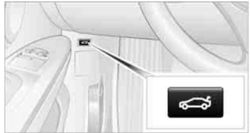
Press the button: the trunk lid opens unless it has been locked.
